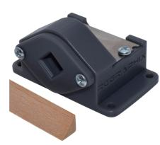
Thank you for your interest in the RG Graphix Balsa Tri-Stock Stripper. This handy tool features a heavy duty blade and comes with four adapters- 1/4", 5/16, 3/8" & 1/2". With these four adapters 1/8", 5/32", 3/16", 1/4", 5/16", 3/8" & 1/2" triangle stock can be produced quickly and easily.
